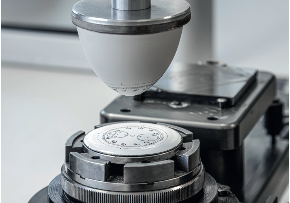
STAMPING THE ENAMEL DIAL WITH MARKINGS
