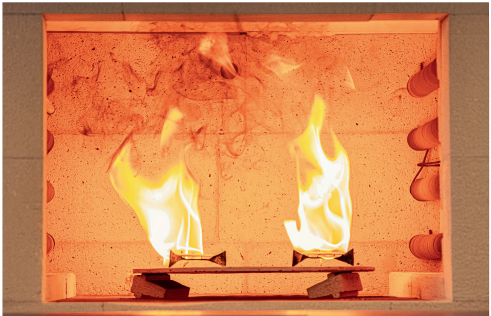
FIRING THE ENAMEL DIAL BASE PLATE IN THE KILN AT 840 DEGREES CENTIGRADE / 1,544 DEGREES FAHRENHEIT
